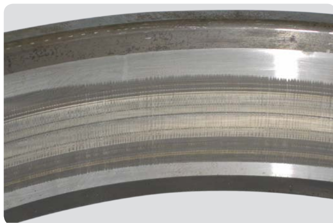
Cylindrical roller bearing outer ring Early stage of washboarding
