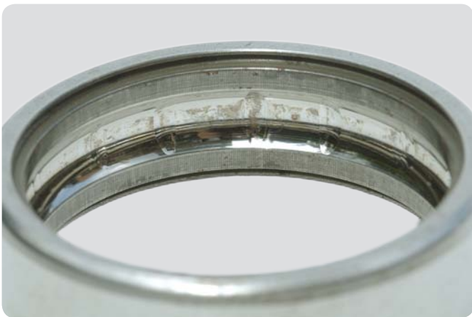
Deep groove ball bearing outer ring Plastic deformation at ball pitch from applying mounting force to the wrong ring
