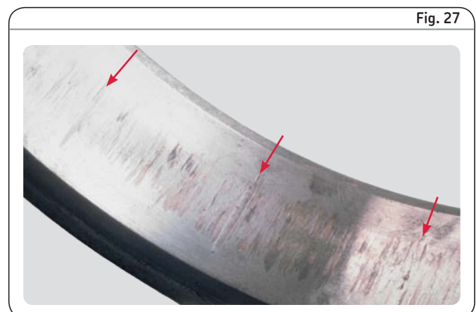
False brinelling (“flutes”) on the outer ring raceway of a cylindrical roller bearing
