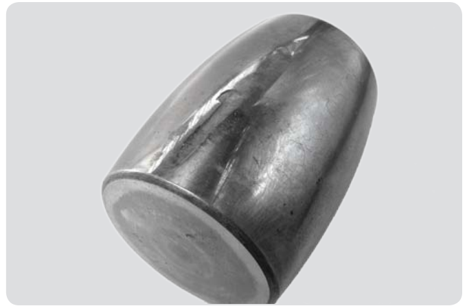
Spherical roller thrust bearing – roller Heavy impact, plastic deformation
