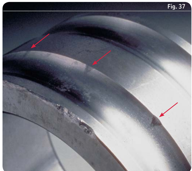
Indentations at ball pitch on the raceway of a double row angular contact ball bearing resulting from incorrect mounting
