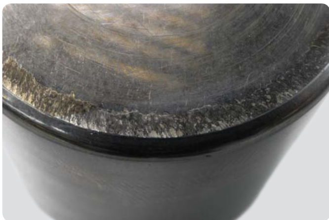
Tapered roller bearing – roller Contamination and inadequate lubrication leading to adhesive wear marks on the large roller end face
