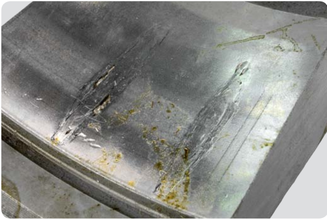
Double row tapered roller bearing outer ring Overload impact and misalignment at standstill, resulting in deformation and subsequent spalling at roller pitch
