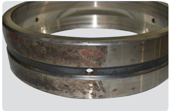
Spherical roller bearing outer ring Inadequately supported ring
