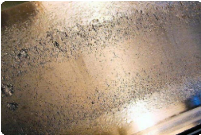
Spherical roller bearing inner ring Inadequate lubrication, surface distress with incipient spalling
