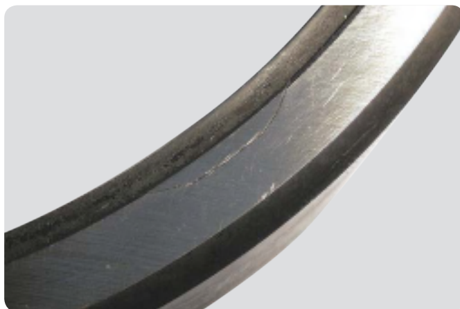
Deep groove ball bearing outer ring side face Fracture at seal anchorage groove due to impact when mounting the bearing
