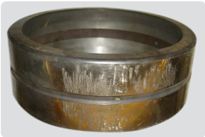
Spherical roller bearing outer ring Brown coloured fretting corrosion area from micromovements due to advanced raceway spalling, with scratches due to dismounting
