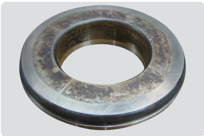
Spherical roller thrust bearing shaft washer Inadequate seat
