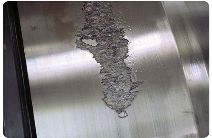
Spherical roller bearing inner ring Material fatigue
