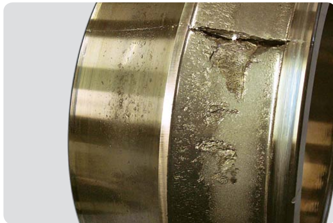
Spherical roller bearing inner ring Very heavy spalling – fatigue fracture as sequential damage
