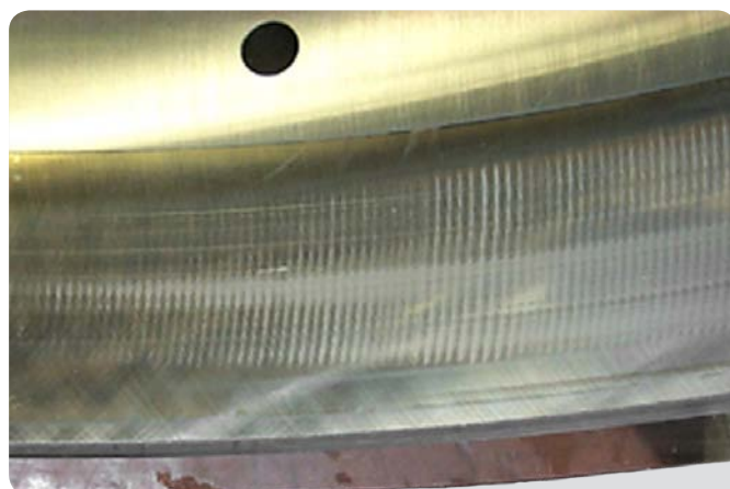
Spherical roller bearing outer ring Current leakage
