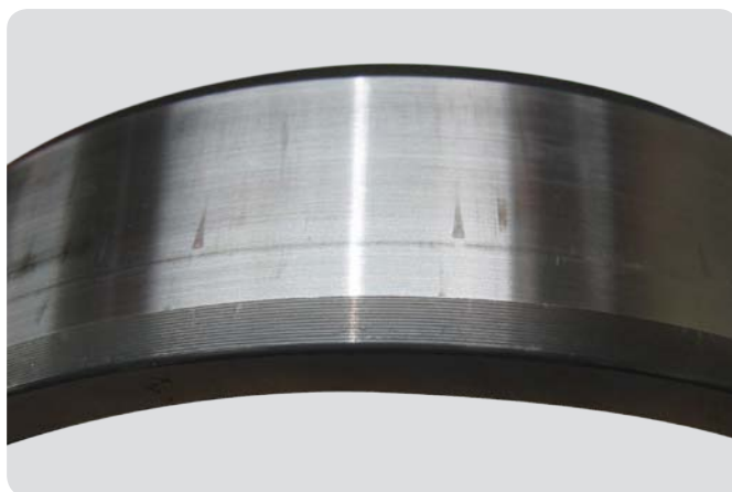
Cylindrical roller bearing inner ring During mounting, inner and outer rings were not aligned properly. Axial marks at roller pitch.
