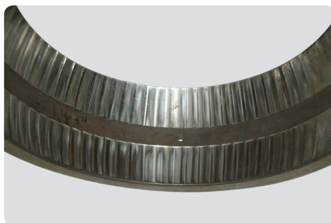
Spherical roller bearing outer ring Exposure to excessive vibrations at standstill, sets of false brinelling marks at roller pitch
