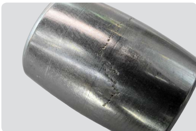
Spherical roller bearing – roller Excessive current resulting in a large number of craters in a zig-zag formation
