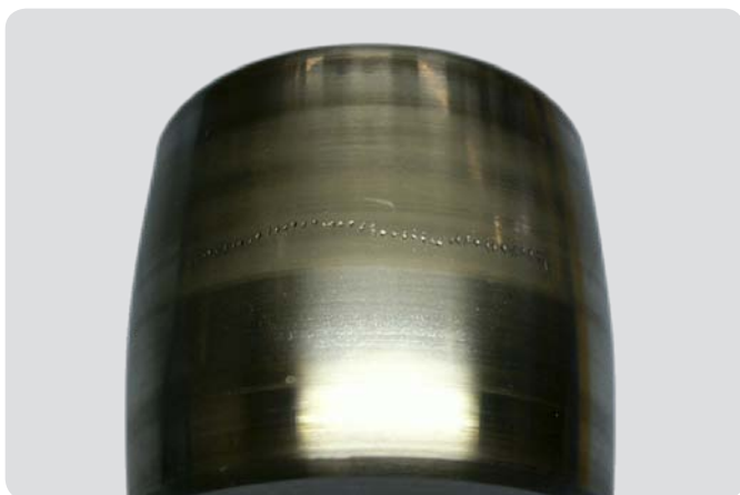
Spherical roller bearing – roller Excessive current resulting in a large number of craters in a bead-like formation
