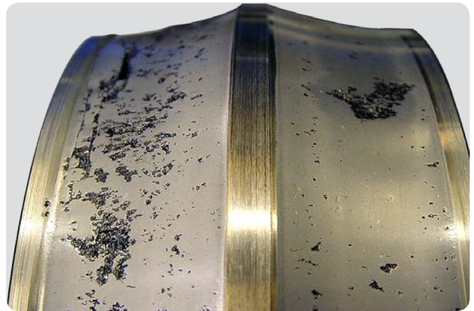
Spherical roller bearing inner ring Inadequate lubricant film. Initially, abrasive wear due to contamination, developed into surface distress and spalling.
