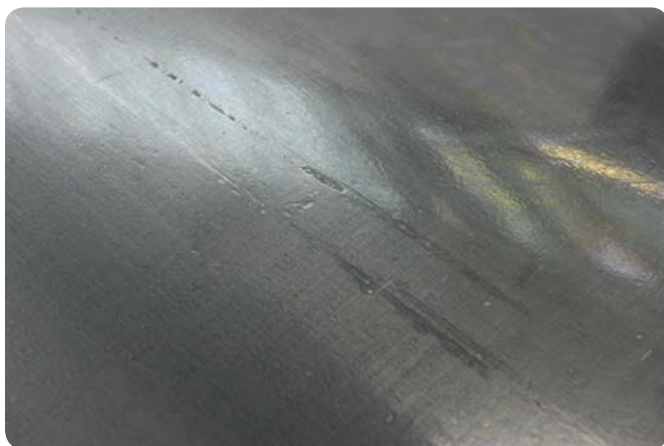
Tapered roller bearing outer ring Scoring during handling
