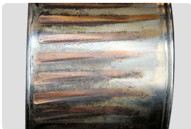
CARB toroidal roller bearing inner ring Exposure to vibrations at standstill with small oscillatory movements, false brinelling marks at roller pitch
