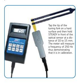
Results within  $\pm 1\%$  are acceptable. There is no adjustment possible. If greater variance is experienced, the meter should be returned for calibration. See section 7.2 for manufacturer's contact information.
