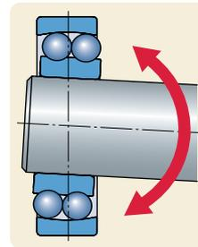
With uneven loads and changes in conveyor belt position, pulley bearings may become misaligned. The chart at left shows the maximum misalignment that can typically be accommodated by various open bearing types. Optimally sized SKF open self-aligning ball bearings can compensate for up to 3 degrees of misalignment, depending on the series.
